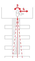
4. Now that the "C" Axis is fixed, you can slide the ring mount pin in the "X" Axis to fine tune the line to final adjustment and tighten.
